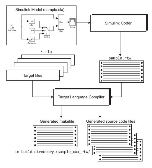
When generating code from a Simulink model, the first step in the automated process is to generate a <code>model.rtw</code> file. The <code>model.rtw</code> file includes the model-specific information required for generating code from the Simulink model. <code>model.rtw</code> is passed to the Target Language Compiler, which uses it in combination with a set of included system target files and block target files to generate the code.
